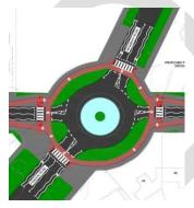
The Dutch-style roundabout designs seek to improve safety for cyclists and pedestrians in a number of ways. One of the key elements is a change in carriageway width, designed to influence slower approach and departure speeds, thereby reducing the speed of drivers.
